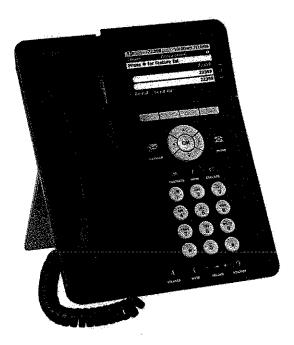
The 9620 IP Telephone features a 3.45 inch (9 cm) diagonal monochrome backlit display - which has been enhanced with higher resolution (1/4 VGA) compared with other available monochrome telephones from Avaya. The 9620 supports up to 12 call appearances and/or administered feature keys - with three concurrent line appearances visible at any time.
