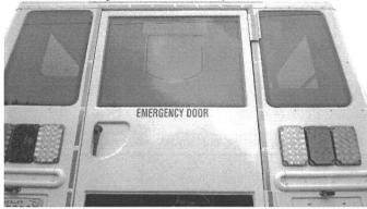
\*rear side corner posts (fasteners are required for manufacturing purposes due to steel structure behind and inability to install rivets)
